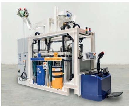
Design example of a NODOPOX for 200 l drums with automated refilling and its own drive unit
